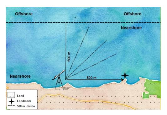
Figure 4. Estimating a distance using a permanent marker.
