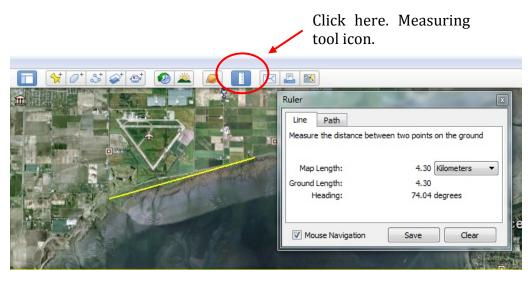
Figure 5. Using Google Earth measuring tool to estimate distance.
